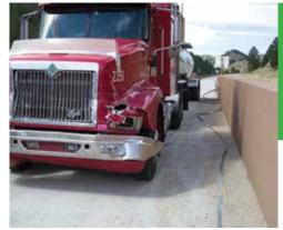
Used CatchNET August 31, 2007. No injuries, minimal damage. 80,000 lbs, 40 mph, used 5 nets.
