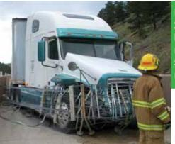
Used CatchNET May 29, 2012. No injuries, minimal damage. 55,000 lbs, 70 mph, used 7 nets.
