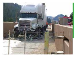
Used CatchNET August 27, 2008. No injuries, minimal damage. 42,000 lbs, 35 mph, used 3 nets.
